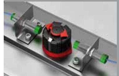
Inductive switches indicating open and closed position
